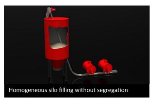
The segregation of bulk materials has consequences on the quality of the final product. Wherever such variations in quality are prohibited, solutions without segregation are required. Complex machinery, such as silo agitators, screw mixers, etc. is often needed.
